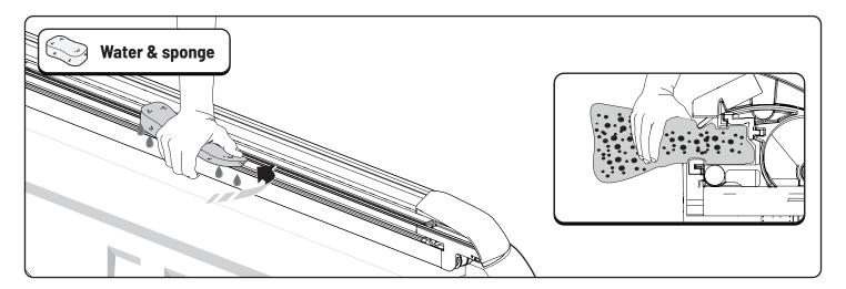
• Clean the drainage channels on the side profiles.
