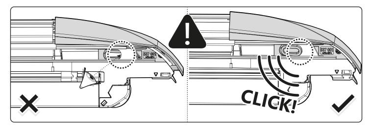
Make sure plastic cover is mounted correctly.
