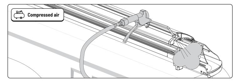
Remove dirt and debris using compressed air.
