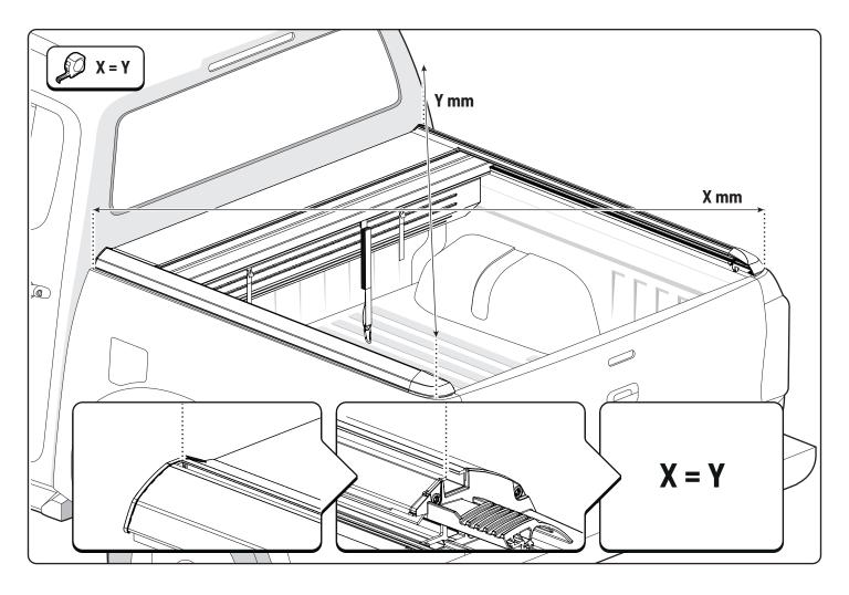
• Ensure the cross measurements are identical.
