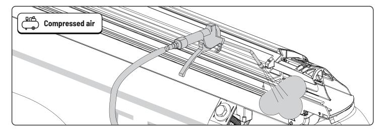
Remove dirt and debris using compressed air.
