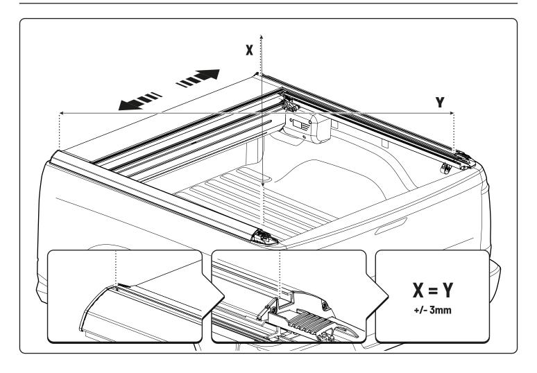
• Ensure the cross measurements are identical.
