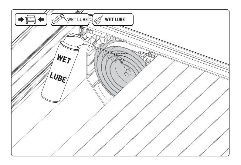
• If your EVOe roll cover has spiral endcaps in the canister, regularly - and following cleaning - apply a PTFE-free all-conditions wet lube product to the inside of the canister ends.
