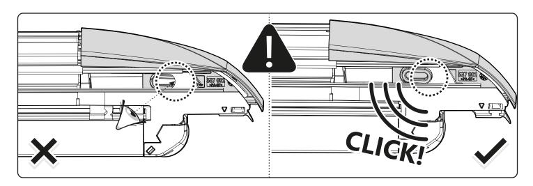
Make sure plastic cover is mounted correctly.
