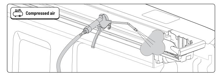
Remove dirt and debris using compressed air.
