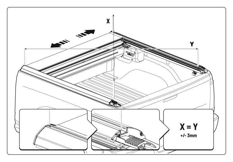
• Ensure the cross measurements are identical.
