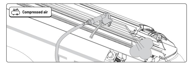
Remove dirt and debris using compressed air.
