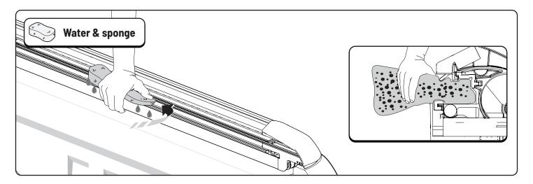
• Clean the drainage channels on the side profiles. Do not use high pressure cleaner.
